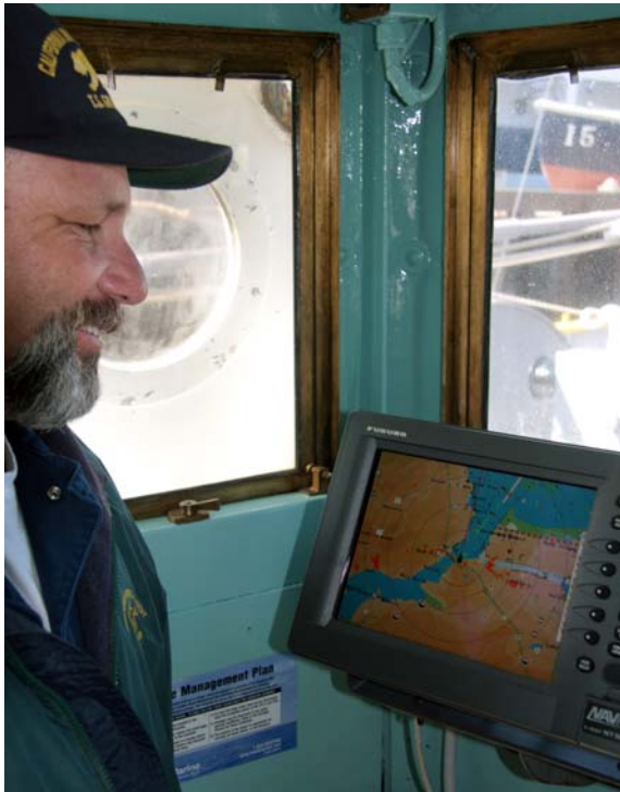
Bob Brown shows off the new radar display unit in the wheelhouse of the work vessel Cub .
